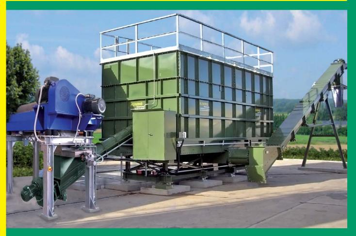
Short loading procedure trough high discharge capacity (typically 27 t in 25 min.)
